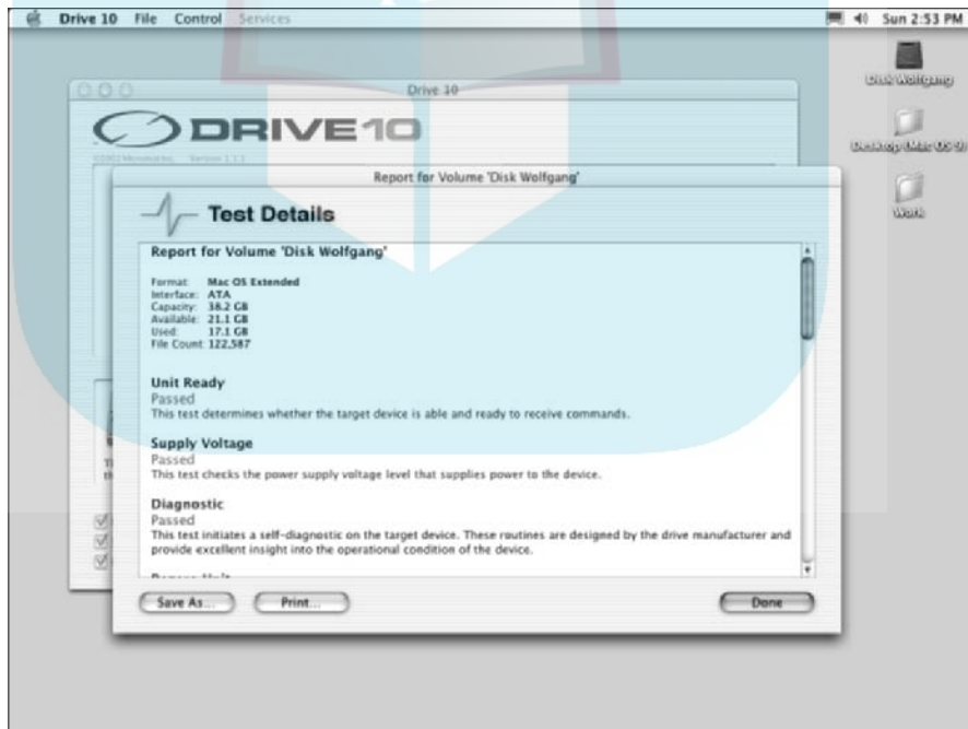
Figure 5-3: Use Drive 10 to check for drive errors.
